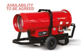
**PHOEN/N:** heavy-duty gas (propane or natural gas) indirect-fired portable heaters with embedded burner with dedicated fan for combustion air. The PHOEN/N heaters feature a heat exchanger that contains the flame and expels fumes throughout a chimney connected to the outside. Being indirect fired, they can be operated indoor and can also be ducted. On the other hand, they have higher upfront costs and about 85% US efficiency due to the heat lost through the chimney.
