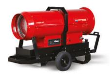
**PHOEN HC:** heavy-duty diesel indirect fired portable heaters with embedded burner with dedicated fan for combustion air. The PHOEN HC heaters feature a heat exchanger that contains the flame and expels fumes throughout a chimney connected to the outside. Being indirect-fired, they can be operated indoor and can also be ducted. On the other hand, they have higher upfront costs and about 85% US efficiency due to the heat lost through the chimney.
