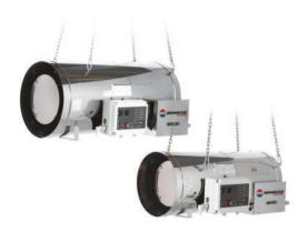
**GA/N:** in stainless steel, can be powered by low-pressure LPG or methane (20-30 mbar), with integrated burner and direct combustion. Can easily be driven by a remote control unit.
