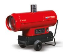
**EC and EC HC:** diesel indirect-fired portable heaters with embedded burner with combustion air obtained from the main ventilation fan. The EC heaters feature a heat exchanger that contains the flame and expels fumes throughout a chimney connected to the outside. Being indirect-fired, they can be operated indoor and can also be ducted. On the other hand, they have higher upfront costs and about 85% US efficiency due to the heat lost through the chimney.
