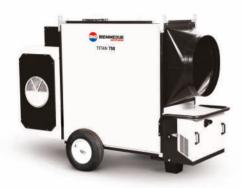
**TITAN:** direct fired heater with considerable size, ideal for large buildings. It features external burner that can be chosen between gas (GPL or natural gas) and diesel. Equipped with centrifugal fan that guarantees low noise operations as well as high static pressure (300 Pa), that makes it suitable in installation with long ducts. The combustion chamber features 5-loop smoke technology to ensure 96% thermal efficiency.
